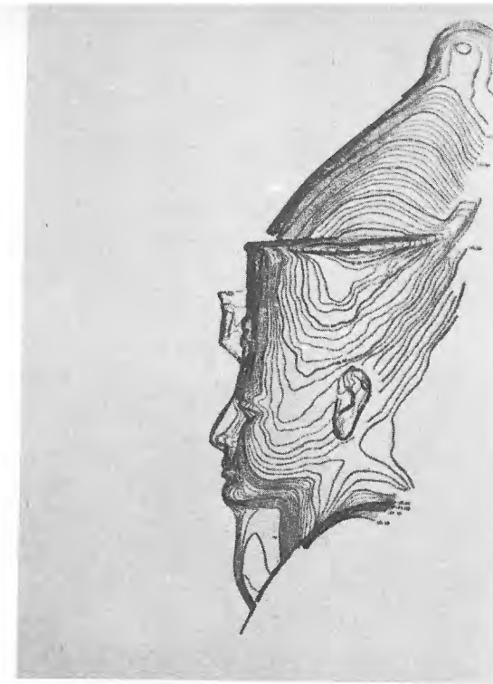
Plate 45. Photogrammetry of the profile of the head of Ramses II (westernmost colossus in the north row, hypostyle hall of the Great Temple at Abu Simbel).
